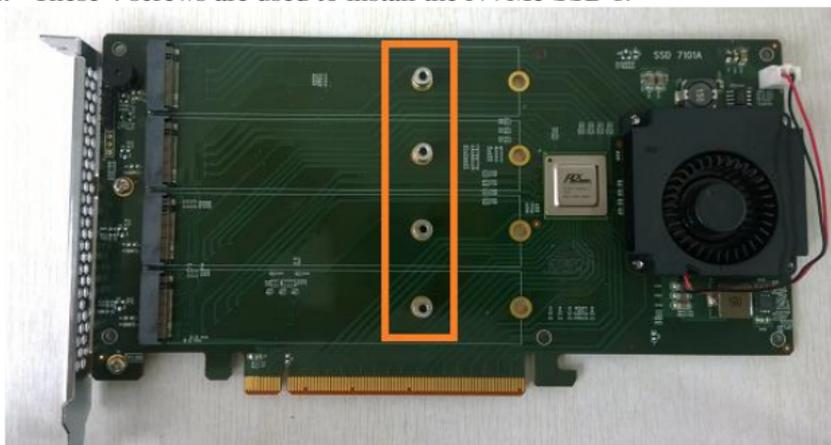
Step 3. The SSDs should be installed from top to bottom. To begin, remove the top screw.
